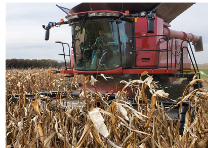
Commercial Combine (8-row) 4 yield monitors (YM1, YM2, YM3, and P1)
