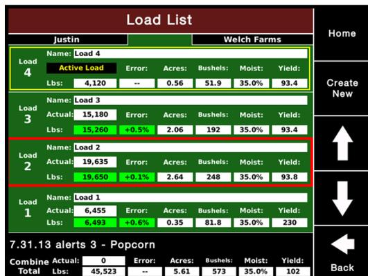
2. When viewing the load list press the box corresponding to the load you want to enter an actual weight for.
