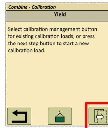
Select the "next" button to begin the first calibration. Ensure that the combine grain tank is empty.
