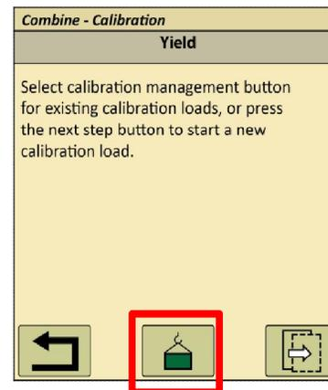
Selecting the "calibration load management" button and be sure to have enough clear calibration loads for the desired number of calibrations you intent to perform at different grain flow rates. Make room by deleting old or unwanted calibration loads.
