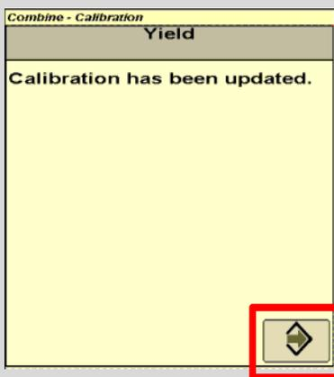
Selecting the "accept" button will complete the weight calibration process.
