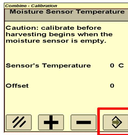
Use the "+" and "-" buttons to accurately identify the offset between the air temperature and the moisture sensor temperature. Change until Sensor's Temperature matches the surrounding temperature.
