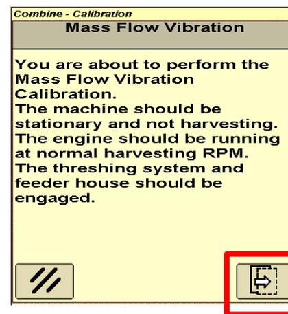
With the combine running and empty of grain, engage the separator and header. While sitting still at full engine RPM and the correct header in the operating position (but not resting on the ground), select the accept button.
