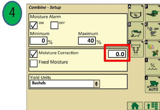
Ensure there is a check mark in the moisture correction box. Then select the correction value, and enter the correct offset between the actual measured value and the displayed value, and accept. This can be a positive or negative number, and needs to be added to any existing offset.
