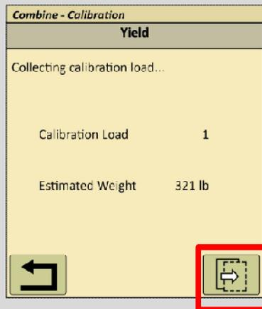
Selecting the "next" button again will complete the calibration load, scale weights will be entered in the calibration management screen
