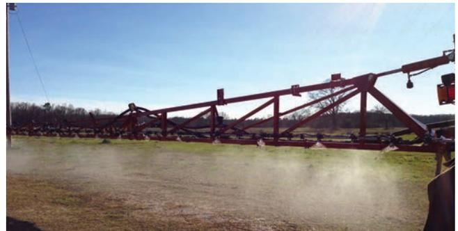
Figure 7. Commercial sprayer with PWM technology
