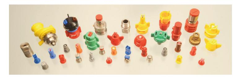
Although nozzles are some of the least expensive components of a sprayer, they hold a high value in their ability to influence sprayer performance. Nozzles meter the amount of liquid sprayed per unit area, controlling application rate, as well as variability of spray over the width of the sprayer boom. Nozzles also influence droplet size, affecting both target coverage and spray drift risk.
